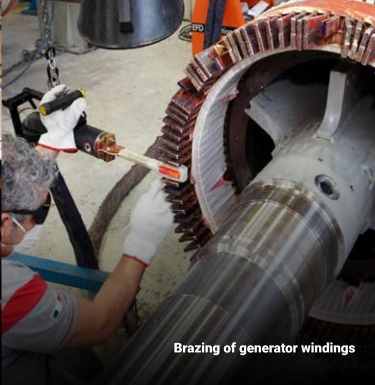
A stationary coil during brazing of a short-circuit ring
