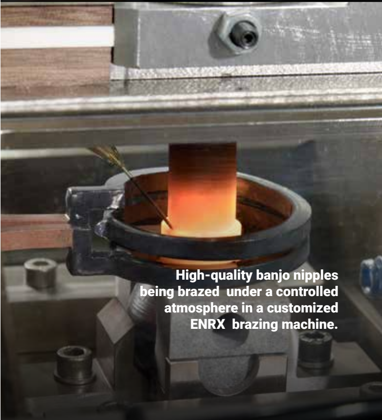
Induction heating is a perfect method for high through-put brazing of evaporator and condenser connections.
