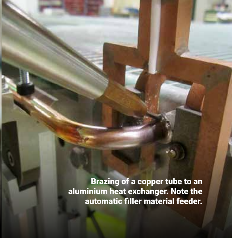
Fast, precise, controllable and easy to use. Induction is perfect for faucet brazing—whether it's tube-to-socket, tube-to-tube or thread insert brazing.
