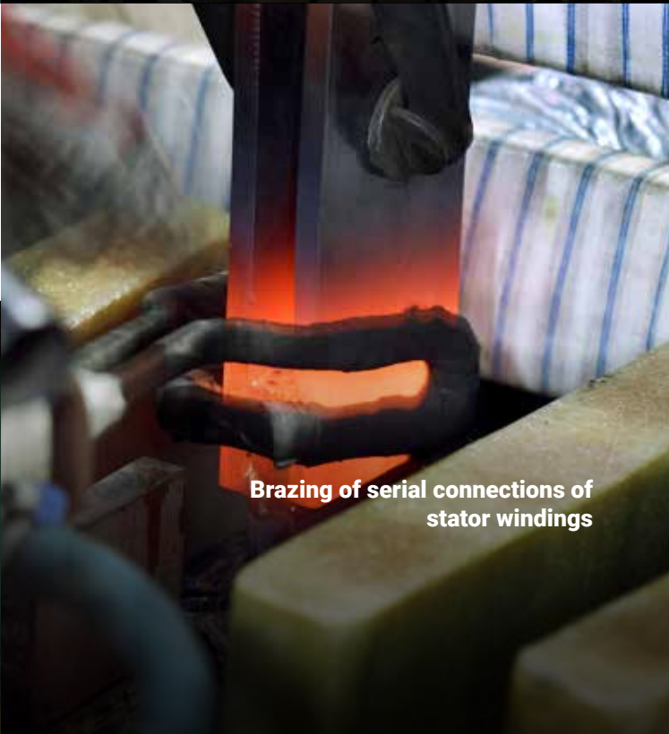
A stationary coil during brazing of a short-circuit ring
