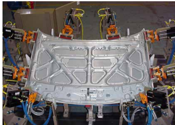
ALUMINIUM HOOD BONDING TOOL: Note the absence of clamps, minimal nest and relatively small curing areas.
